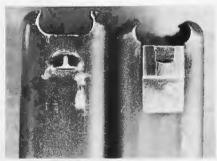
Canadian FAL magazine (right) has durable solid-metal front lug which — unlike punched standard mag lug on left — needs no special care or inspection.
